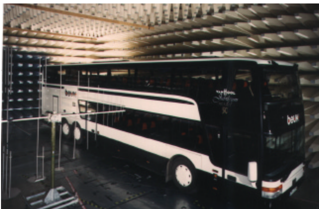
Immunity test of a Bus in the anechoic chamber
